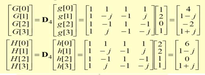
$$\mathbf{Y}_{C}[k] = \begin{bmatrix} Y_{C}[0] \\ Y_{C}[1] \\ Y_{C}[2] \\ Y_{C}[3] \end{bmatrix} = \begin{bmatrix} G[0]H[0] \\ G[1]H[1] \\ G[2]H[2] \\ G[3]H[3] \end{bmatrix} =$$
